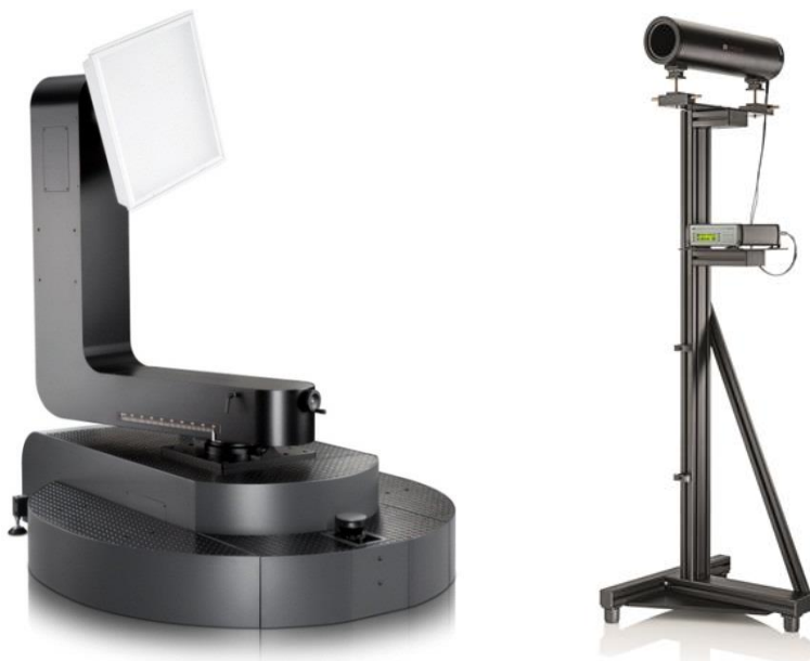
Image 2: Turning luminaire goniometer (left) and measuring probe enclosed in the stray light tube on a stand (right).
