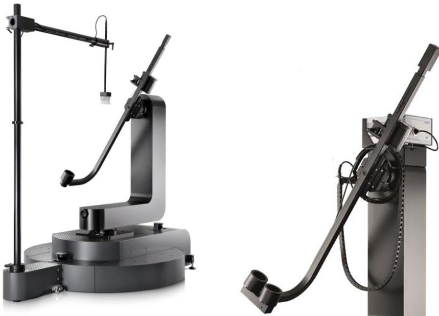
Image 3: Goniophotometer luminous flux integrator (left) and luminous flux integrator with photometer and spectroradiometer (right).
