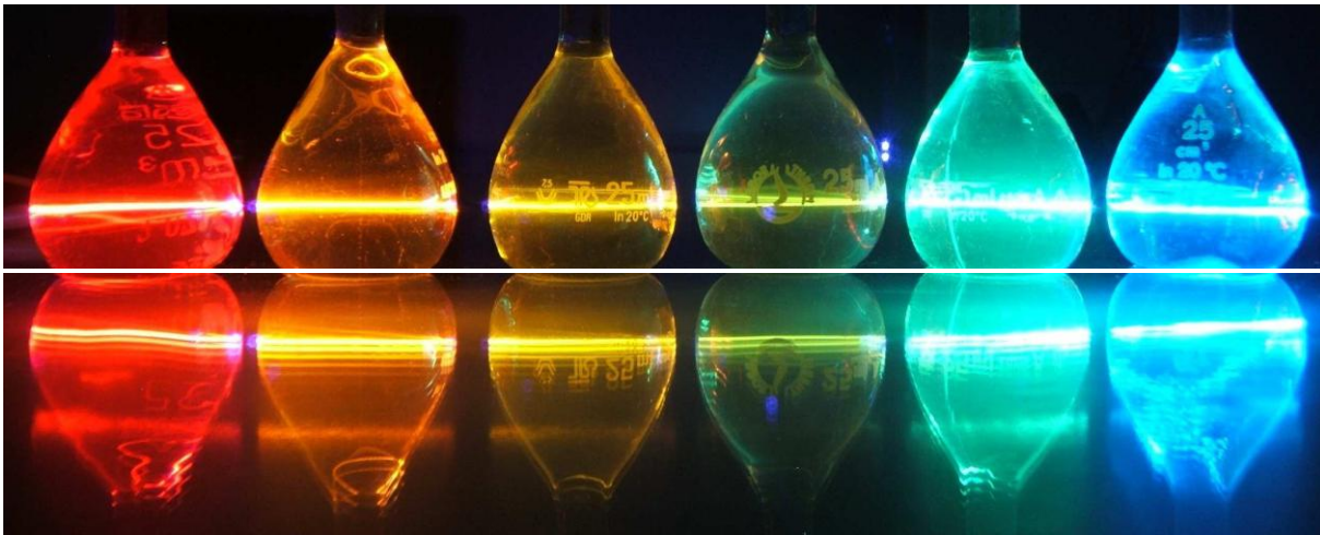
Excitation of multiple fluorophores by using a single 405 nm diode laser module of the LASOS ® LDM laser series
