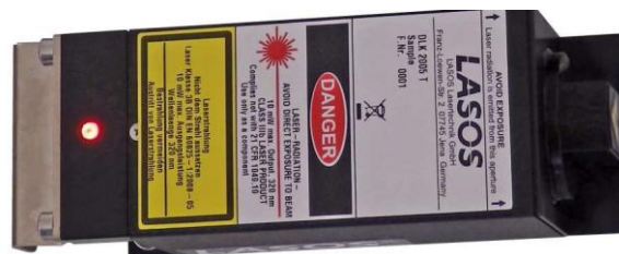
Compact diode-pumped solid-state laser emitting at 320 nm
