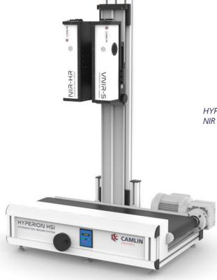
HYPERION HSI system configured with dual camera mount (VNIR and NIR cameras) and conveyor scanning stage. On/off rollers not shown
