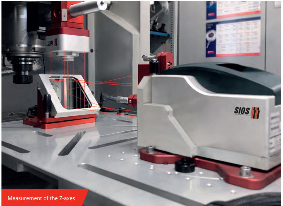
Compact measurement on a high-precision machine tool
