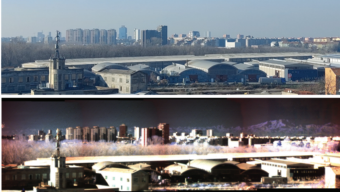
This remote landscape hyperspectral image has been obtained by acquiring three separate hyperspectral images with HERA eSWIR, which have been stitched together during data analysis.
